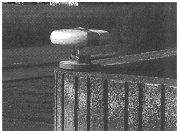
Figure 1: Dual-frequency GPS/Glonass receiver and antenna at Delft University of Technology. The receiver is connected to a PC for real-time integrity monitoring of the data.
